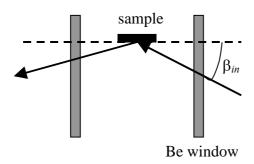
The first case occurs when the glancing X-ray beam traverses a sample chamber, liquid column etc. in the perpendicular direction. The figure shows how the path length traversed by the X-rays depends on the incoming or outgoing angles. We discuss here only the incoming beam, the exit beam is completely analogous. For incoming angle equal to zero  $(\beta_{in}=0)$ , the transmission is equal to:
