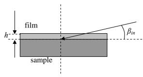
For the second case, the path length traversed is determined by the perpendicular thickness of a film (or other material) on top of surface/interface (see figure). The transmission through the film in the perpendicular direction is:
